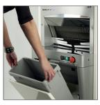
Removable crumb collector Accessible by tilting the front, cylinder-assisted door. 4.7 gallons capacity.
